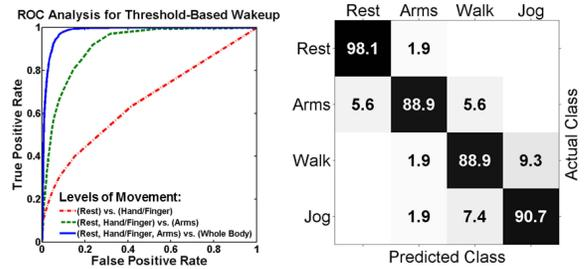
Figure 4. Left: ROC curves for threshold-based wake-up. Right: Confusion matrix of motion type classification.
