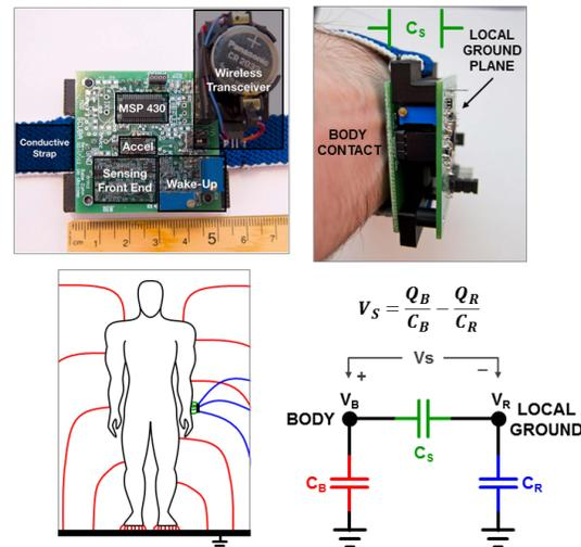
Figure 1. Static EF sensing utilizes capacitive coupling between the body, the sensor's local ground plane, and the environment. *Top Left*: Prototype sensing platform. *Top Right*: Side view of sensor platform showing spacing between the body and the local ground plane. *Bottom Left*: Capacitive coupling indicated by field lines, closer lines indicate stronger coupling. *Bottom Right*: Circuit model of sensing technique.
