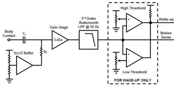
Figure 3. Block diagram of hardware for motion sensing.
